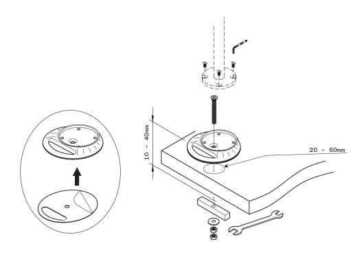
Adhesive the pad under the grommet mount. Use large bolt to go thru parts (see figures) Desk thickness from 10mm~40mm. Advise for desk thickness above 30mm. The diameter of the hole is from 20mm to 60mm.
