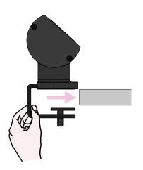
**FASTEN CLAMP** Use 4 mm Allen key to tighten the hexagon cup point screw. Turn clockwise to tighten and ascertain that the product does not move if pushed or pulled.
