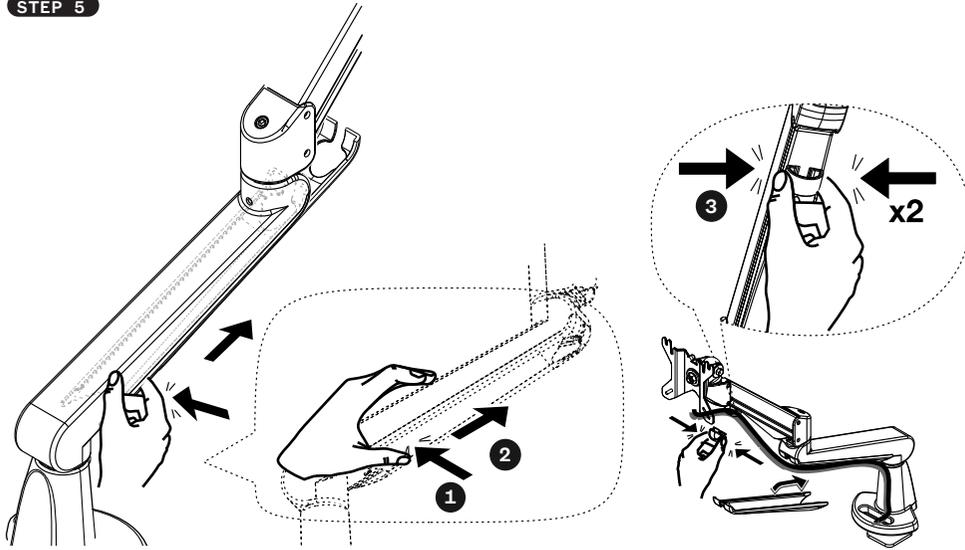
Unattach the cable collector and route the cables through. Once satisfied, re-attach the collector back into place. Proceed by continuing the routing through the cable clip.
