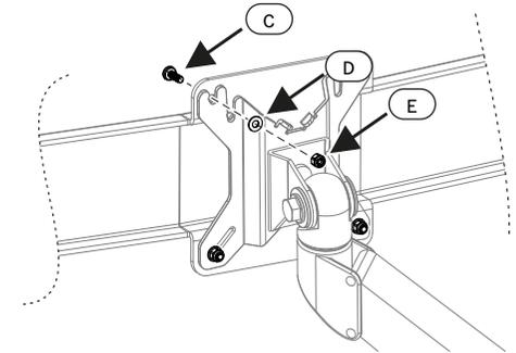
Place the LCD monitor face down on a flat surface. Align the VESA on a flat surface. Align the VESA bracket (B) holes and fasten using screws (C). Repeat procedure for both LCD monitors.
