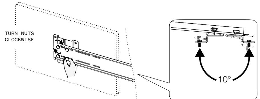
Lift the VESA bracket with the mounted LCD monitor, and examine how close the monitor can be to the center of the bar (see step 6). Then, insert the VESA bracket pins into the track of the bar and lock them to the track using the knob nuts (F). Angle the monitor as you see fit. Repeat procedure for both VESA brackets.
