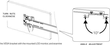
Lift the VESA bracket with the mounted LCD monitor, and examine how close the monitor can be to the center of the bar (see step 6). Then, insert the VESA bracket pins into the track of the bar and lock them to the track using the knob nuts (F). Angle the monitor as you see fit. Repeat procedure for both VESA brackets.
