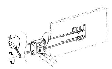
Use 14 mm wrench to tighten the bar to a vertical position. Hold it up to the desired position and use the VESA bracket or Duo Bar as a gripping surface to counter the force of the wrench and gravity.
