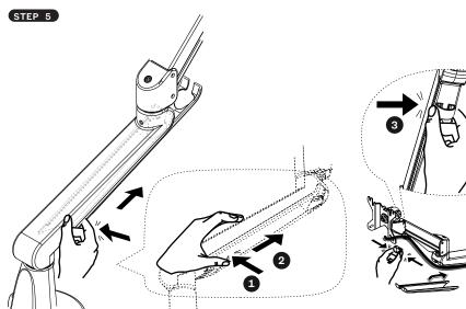
Unattach the cable collector and route the cables through. Once satisfied, re-attach the collector back into place. Proceed by
