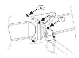
Place the LCD monitor face down on a flat surface. Align the VESA on a flat surface. Align the VESA bracket (B) holes and fasten using screws (C). Repeat procedure for both LCD monitors.
