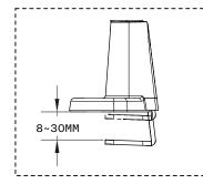
Turn grommet upside down and adhere the Pad (B). Use Allen Key (H) to adjust the height of the clamp so that it fits your table. Tighten until sturdy and ascertain that the clamp can not be moved from its position from the table.
