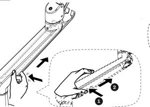
Unattach the cable collector and route the cables through. Once satisfied, re-attach the collector back into place. Proceed by continuing the routing through the cable clip.
