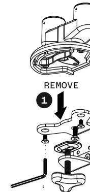
Use the same three screws to fasten the In-Desk bracket (B) and long bolt (D).
