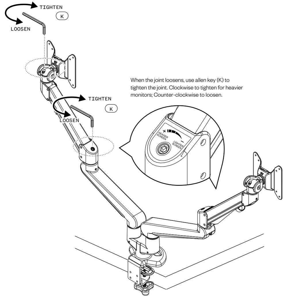
When the joint loosens, use allen key (K) to tighten the joint. Clockwise to tighten for heavier monitors; Counter-clockwise to loosen.
