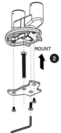
Adhere pad (A1) to the bottom of the clamp, through the long bolt. Insert the re-assembled clamp through the hole in the table. Secure the clamp using all remaining parts F, G, E, N. Be sure to tighten both nuts.
