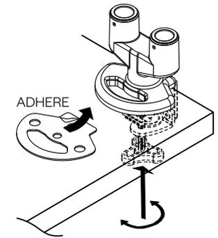
\*Adhere pad (A1) to the bottom side of the clamp (A2). Fasten clamp to the table using the handle. Consider re-positioning the clamp bracket in accordance to the table thickness using the guidelines below.
