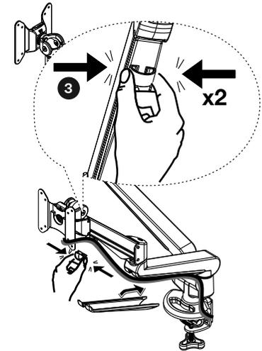
Unattach the cable collector and route the cables through. Once satisfied, re-attach the collector back into place. Proceed by continuing the routing through the cable clip.
