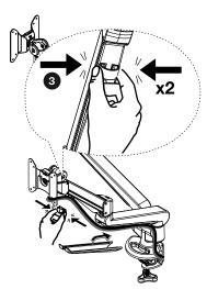
Unattach the cable collector and route the cables through. Once satisfied, re-attach the collector back into place. Proceed by continuing the routing through the cable clip.
