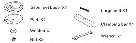
Adhesive the pad under the grommet mount. Use large bolt to go thru parts (as figures blow). Desk thickness from 10mm~40mm. Advise for desk thickness above 30mm. The diameter of the hole is from 20mm to 60mm.
