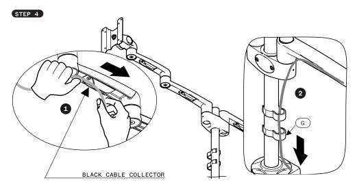
Finish installation by directing the cables from the monitors through both black cable collectors. Lastly, direct the cable further down the pole and attach all cable clips to keep them in place.
