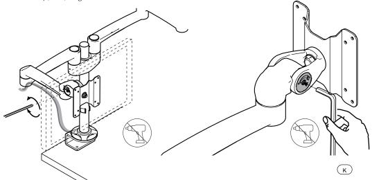
Weight capacity for ~14kg monitors. Loading capacity could be reduced if the monitor size is greater than 26 inches or if the thickness exceeds 5,5 cm.
