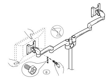
Mount both monitors to the VESA brackets with the provided screws.
