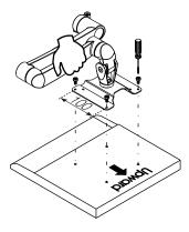
Attach the monitor arm (G) to the LOD monitor using all four screws (H)
