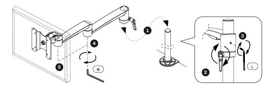
Insert the arm with the fixed LCD monitor onto the pole. Adjust to desired height using the black plastic lever. To make the first arm completely rigid, use Allen key (L) until the screw grips the pole (C). Using Allen key (M), tighten the remaining joints to achieve the same result.
