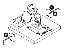
Use Allen key (M) to loosen the left screw completely. Then, tighten the right screw to max torque. Adjust the angle of the LCD and secure its position by re-tightening the screw to max torque. The joint should now be completely rigid.
