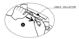
Finish installation by directing the cables from the LCD monitor through both black monitor arm collectors, and finally both cable clips (I) as illustrated below.
