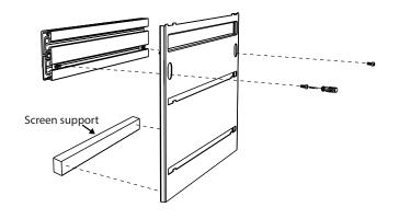
Attach the shelves 2 to the hanger 1 starting from the bottom. Fit the holes with the flaps of the hanger and repeat until fully assembled.
